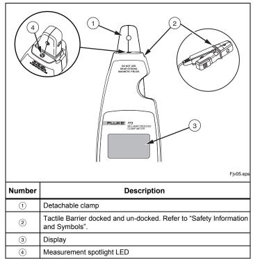
Figure 2. The Milliamp Process Clamp Meter
