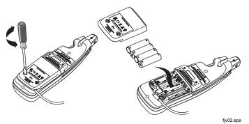
Figure 11. Changing the Batteries
