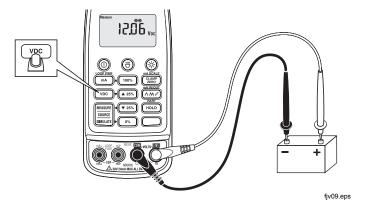
Figure 7. Taking Measurements with the Test Leads
