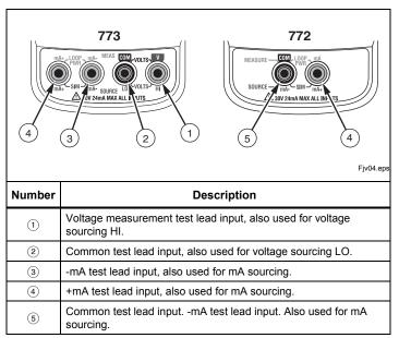
Figure 4. Input/Output Jacks
