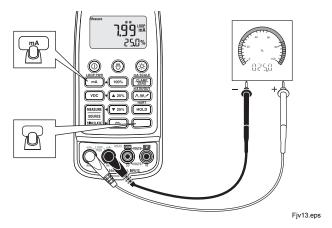
Figure 10. Using Loop Supply Mode
