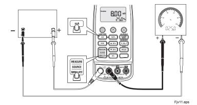
Figure 9. Simulating mA Output
