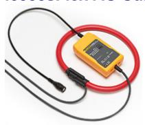
The i6000sflex is an AC current probe utilising the Rogowski principle. It can be used to measure currents up to 6000A when used in conjunction with oscilloscopes, recorders or data loggers. The flexible and lightweight measuring head allows guick and easy installation in hard to reach areas.
