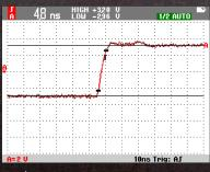
5GS/s sampling or 200 ps sample resolution provides the detail needed to inspect signal edge dV/dt or signs of destructive reflections.
