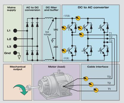
In three-phase systems like variable speed drives, UPS or back-up generators, use four channels to diagnose power input, dc to ac converters, or cable interface problems.
