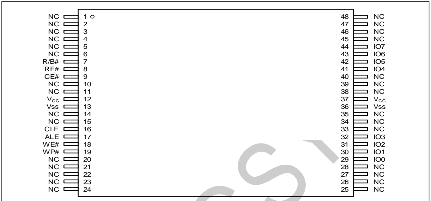
Figure 2 Pin Configuration 48-TSOP
