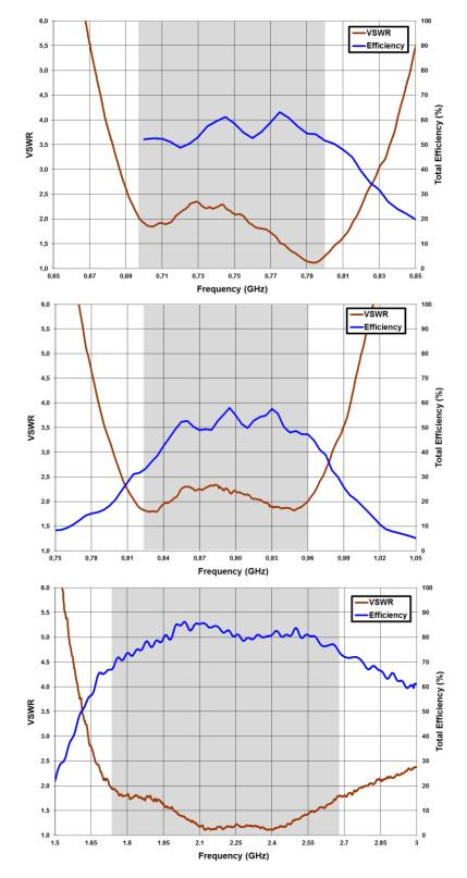
**Figure 3 –** VSWR and Total Efficiency for the 698 – 798 MHz range, for the 824 – 960 MHz range, and for the 1710 – 2690 MHz range from the Evaluation Board 3 ports (Figure 1).
