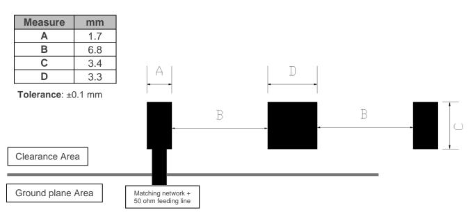
Figure 10 – Footprint dimensions for the double booster.
