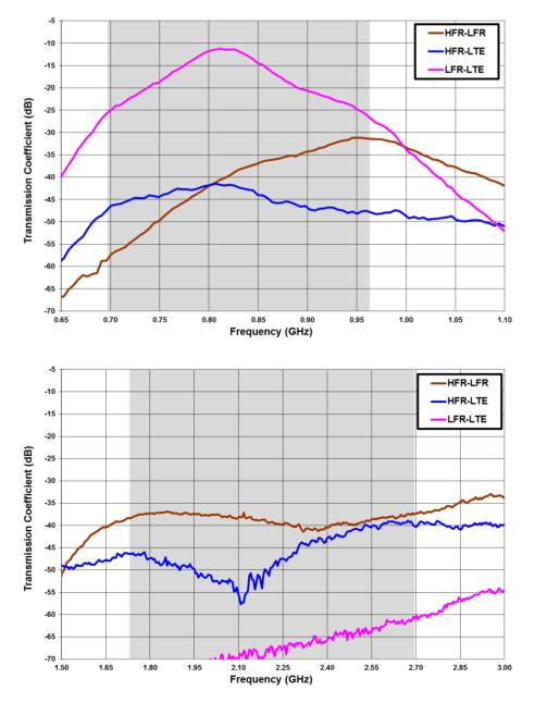
**Figure 4 –** Transmission coefficient for the 698-798 MHz range (LTE), for 824 – 960 MHz range (LFR), and for the 1710 – 2690 MHz range (HFR) (from the Evaluation Board 3 ports) (Figure 1).
