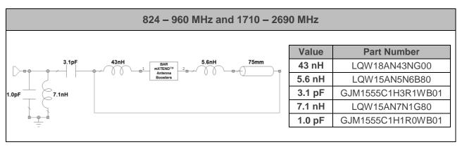
Figure 6 – Matching network implemented in the Evaluation Board 1 port (Figure 5).
