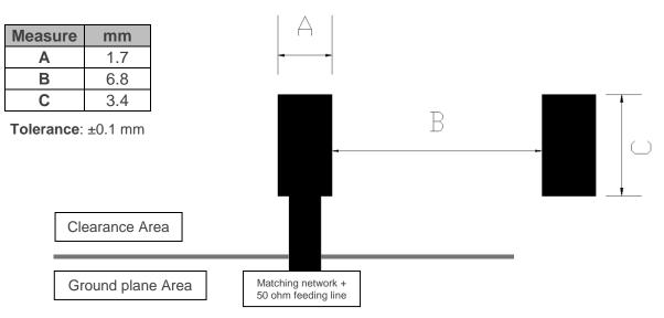
**Figure 9 –** Footprint dimensions for the single booster.
