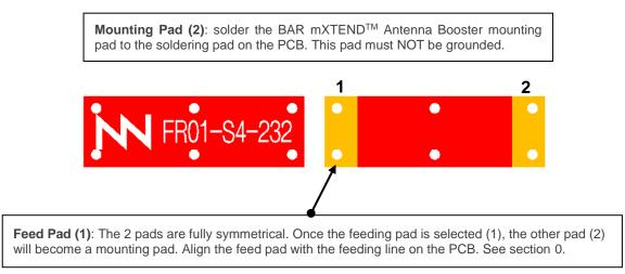
Figure 11 – Pads of the BAR mXTEND<sup>™</sup> Antenna Booster FR01-S4-232.
