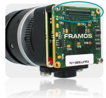
Note: SLVS-EC and SLVS operation modes share partially the same pins. The numbering of D\_DATA\_n pins is applied according to SLVS-EC. For SLVS operation, please refer to Chapter 4.1.3.
