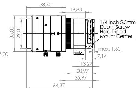
Note: Sensor image optical center is in mechanical board center.
