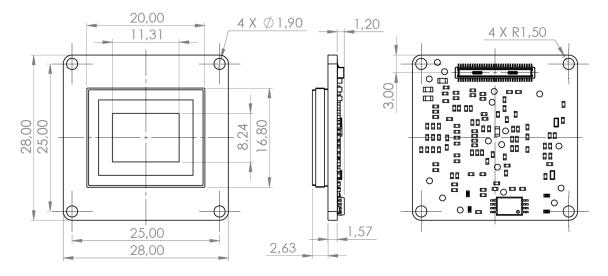
Sensor image optical center is in mechanical board center.
