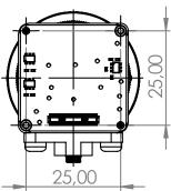
Connector Pinout Module: FSA-FT18/BC Type: Hirose DF40C-60DP-0.4V(51) Label: J1
