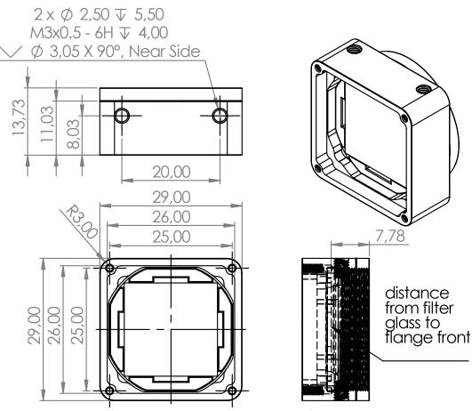
Figure 4: CS-Mount Body for 28 mm FSM
