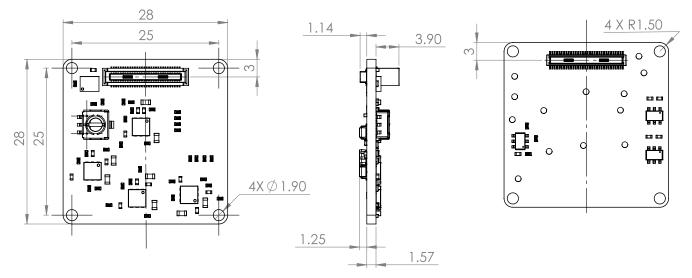
Figure 1: Technical Drawing of FSA-FTx/BC-V1
