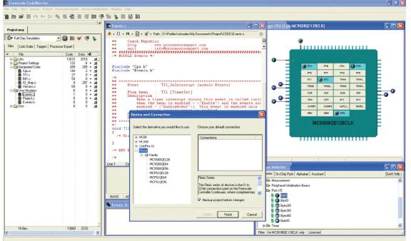
appropriate support files (header files, libraries and linker files). For projects switching between 8-bit and 32-bit Flexis™ series microcontrollers this is the extent of the porting effort.
