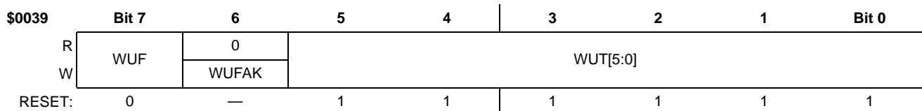
Figure 62. PWU Control/Status Register 0 (PWUCS0)
