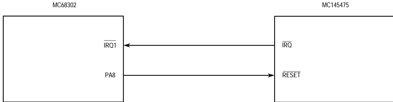
Figure D-17. Discrete Signal Interconnection
