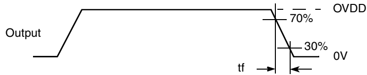
Figure 7. Definition of Timing for Standard and Fast-Mode
