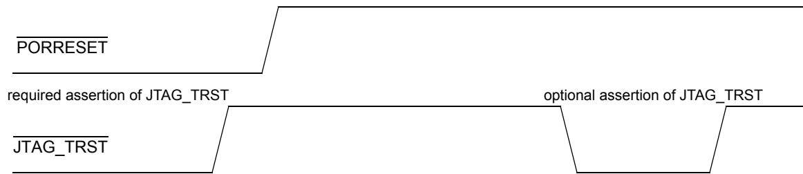
Figure 54. \overline{\text{PORRESET}} vs. \overline{\text{JTAG\_TRST}}
