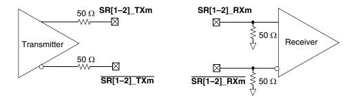
**Note:** The [1–2] indicates the specific SerDes Interface (1 or 2) and the m indicates the specific channel within that interface (0,1,2,3). Actual signals are assigned by the HRCW assignments at reset (see **Chapter 5**, *Reset* in the reference manual for details)
