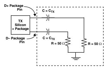
Figure 19. SGMII AC Test/Measurement Load
