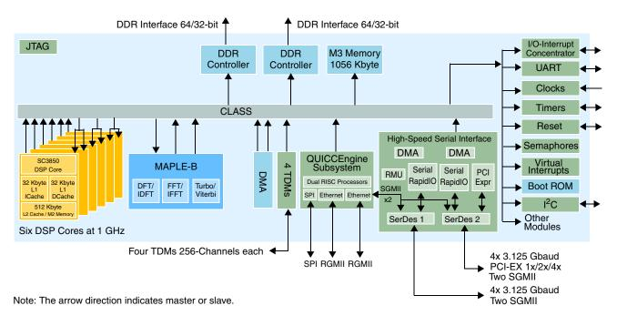
Figure 1. MSC8156 Block Diagram
