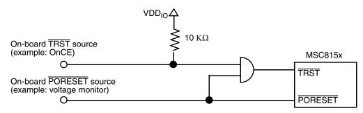
Figure 36. Reset Connection in Debugger Application
