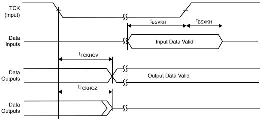
Figure 30. Boundary Scan (JTAG) Timing
