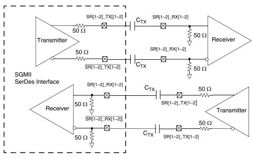
Figure 39. 4-Wire AC-Coupled SGMII Serial Link Connection Example
