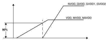
Figure 34. Supply Ramp-Up Sequence
