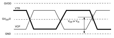
Figure 15. DDR2 and DDR3 SDRAM Differential Timing Specifications
