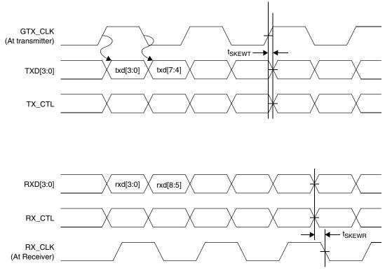
Figure 25. RGMII AC Timing and Multiplexing
