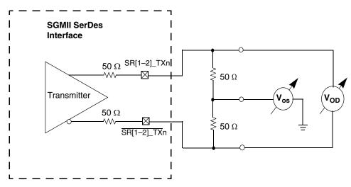
Figure 10. SGMII Transmitter DC Measurement Circuit
