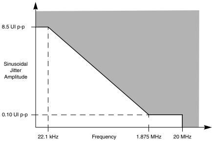
Figure 18. Single Frequency Sinusoidal Jitter Limits
