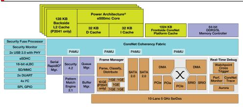
Core Complex (CPU, L2 and Frontside CoreNet Platform Cache) Accelerators and Memory Control
