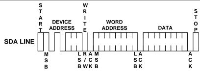
Figure 5: Byte Write
