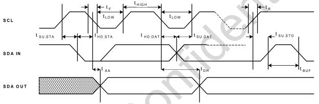
Figure 10: SCL and SDA Bus Timing
