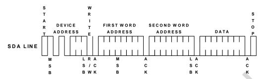
Figure 5: Byte Write
