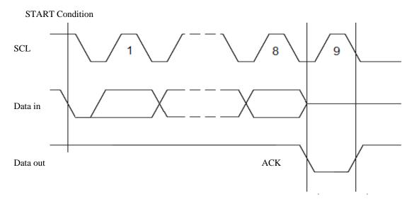
Figure 2: Timing diagram for output ACKNOWLEDGE
