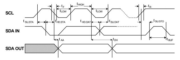
Figure 8: SCL and SDA Bus Timing
