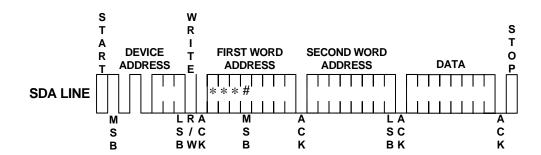
Figure 3: Byte Write
