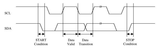
Figure 1: Timing diagram for START and STOP conditions
