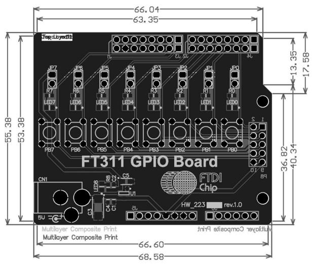
Figure 3.1: FT311 GPIO Board Layout
