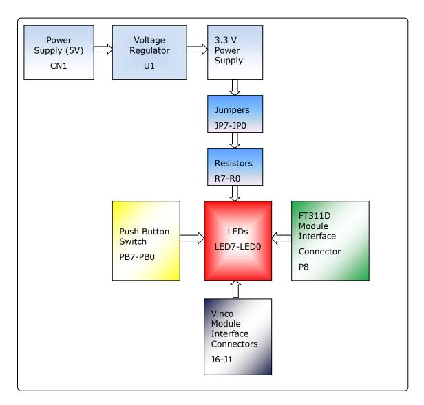
Figure 2.1: FT311 GPIO Board Block Diagram
