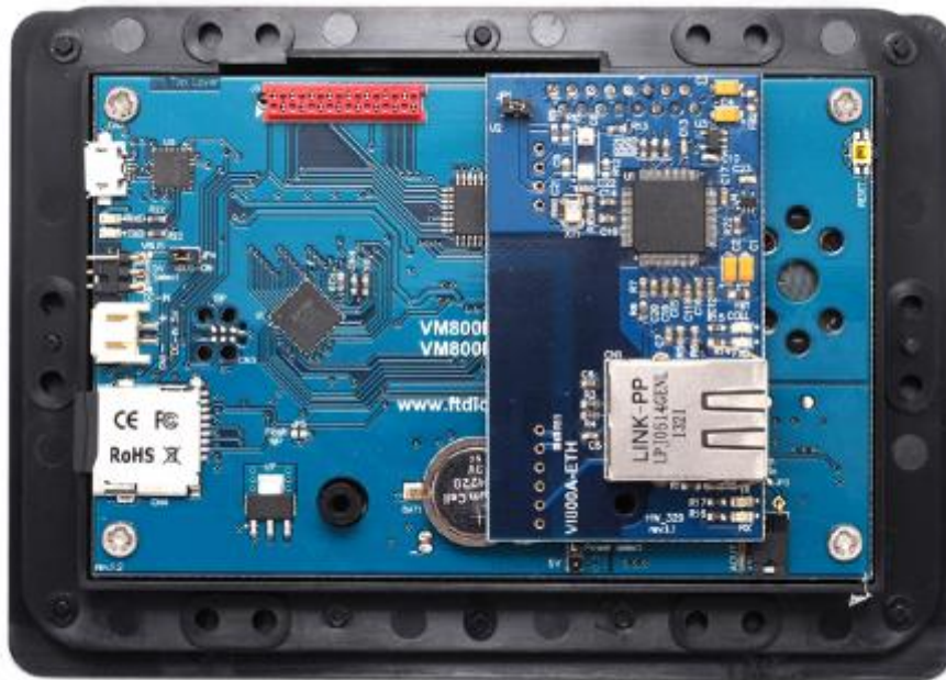
Figure 6-1 – VI800A Ethernet module connected to VM800P Plus module
