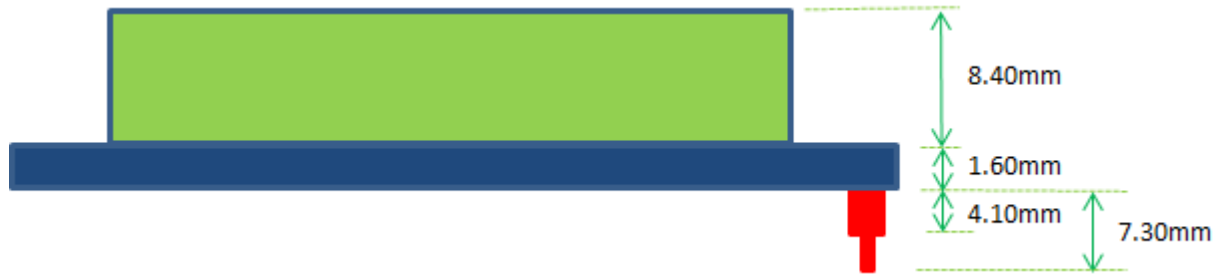
Figure 3-4 - VI800A-N485U module PCB side view
