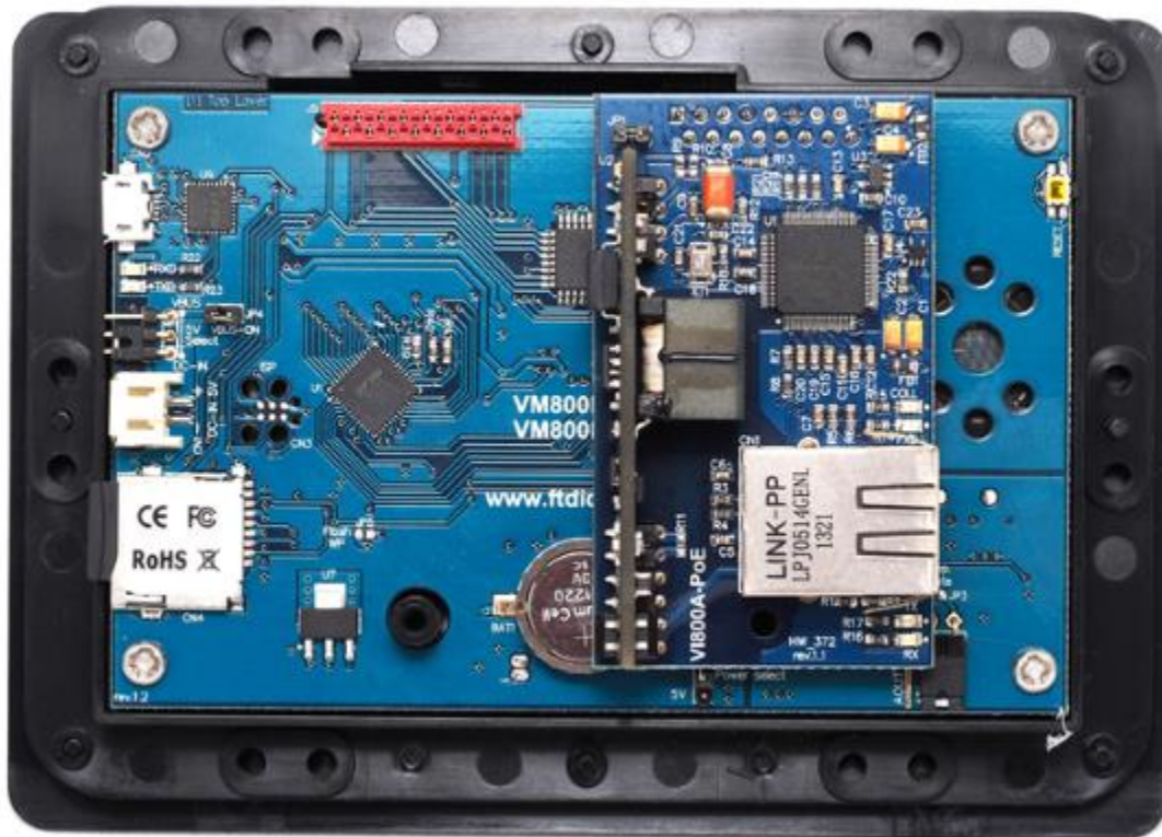
Figure 5-1 – VI800A-PoE module connected to VM800P Plus module
