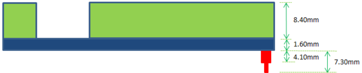
Figure 3-4 - VI800A-RELAY module PCB Side view
