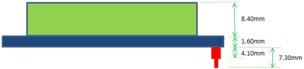
Figure 3-4 - VI800A-TTLU module PCB Side view
