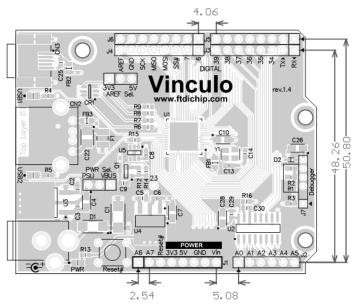
Figure 8.2 - Vinculo Pitch Measurements
