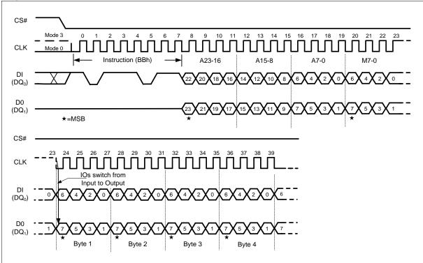
Figure 23 Fast Read Dual I/O Instruction (Initial instruction or previous M5-4 ≠ 10, SPI Mode only)
