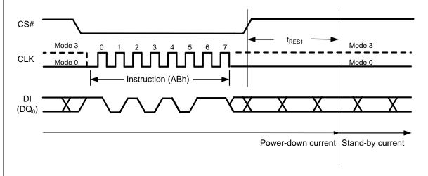
Figure 45 Release Power-down Instruction (SPI Mode)
