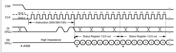
Figure 12 Read Status Register Instruction (SPI Mode)
