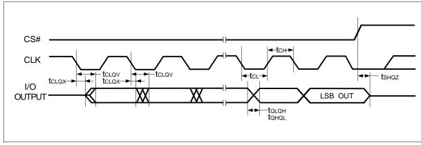
**Figure 74 Serial Output Timing**
