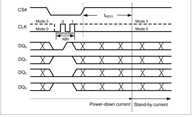
Figure 46 Release Power-down Instruction (QPI Mode)
