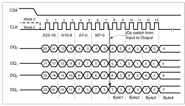
Figure 31 Octal Word Read Quad I/O Instruction (Previous instruction set M5-4 = 10, SPI Mode only)
