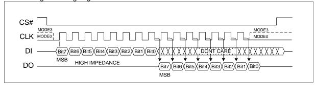
Figure 3 The difference between Mode 0 and Mode 3
