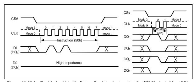
Figure 10 Write Enable for Volatile Status Register Instruction for SPI Mode (left) or QPI Mode (right)
