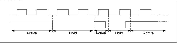
Figure 4 HoldCondition Waveform
