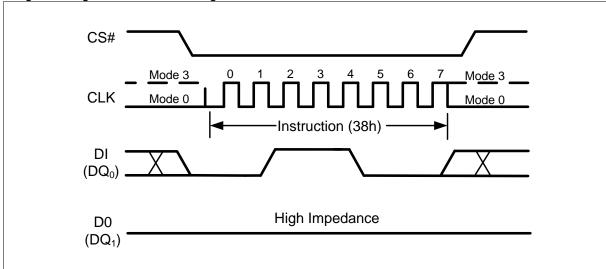
Figure 68 Enable QPI Instruction (SPI Mode only)
