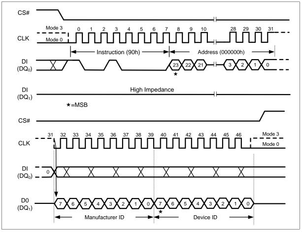
Figure 49 Read Manufacturer / Device ID Instruction (SPI Mode)
