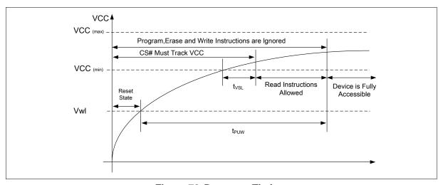
Figure 72 Power-up Timing
