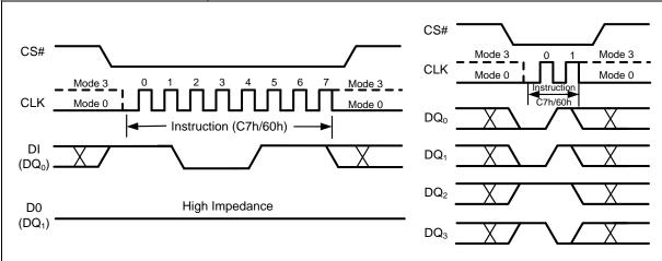
Figure 42 Chip Erase Instruction for SPI Mode (left) or QPI Mode (right)
