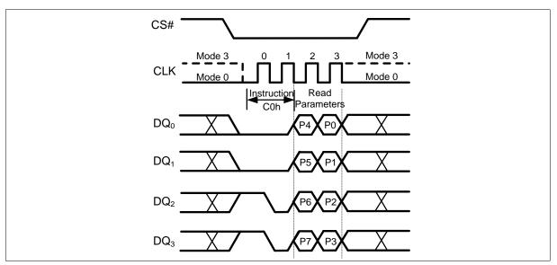
Figure 61 Set Read Parameters Instruction (QPI Mode only)
