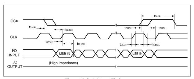
Figure 75 Serial Input Timing
