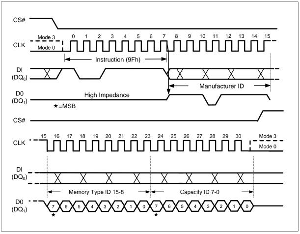
Figure 54 Read JEDEC ID Instruction (SPI Mode)
