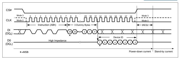
Figure 47 Release Power-down / Device ID Instruction (SPI Mode)
