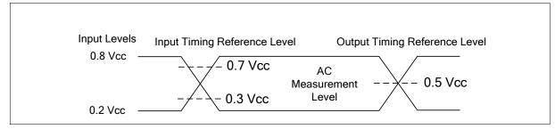
Figure 73 AC Measurement I/O Waveform
