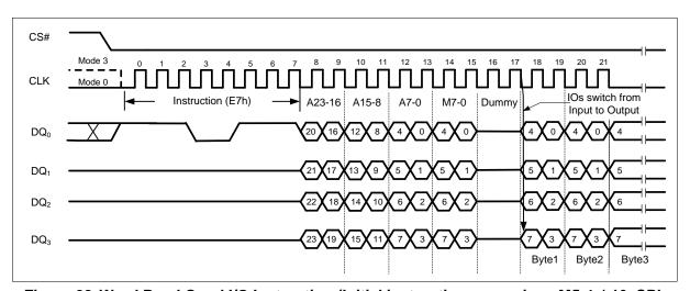
Figure 28 Word Read Quad I/O Instruction (Initial instruction or previous M5-4 ≠ 10, SPI Mode only)
