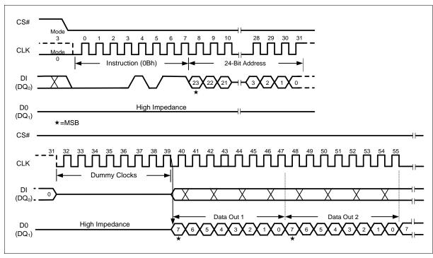
Figure 19 Fast Read Instruction (SPI Mode)
