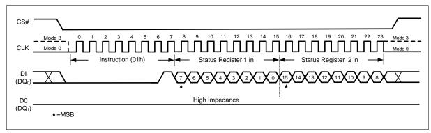
Figure 16 Write Status Register-1/2 Instruction (backward compatible, SPI Mode)
