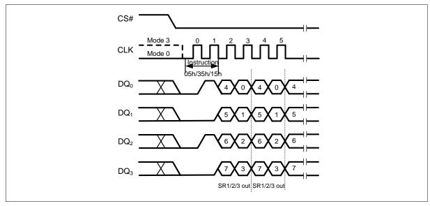
Figure 13 Read Status Register Instruction (QPI Mode)
