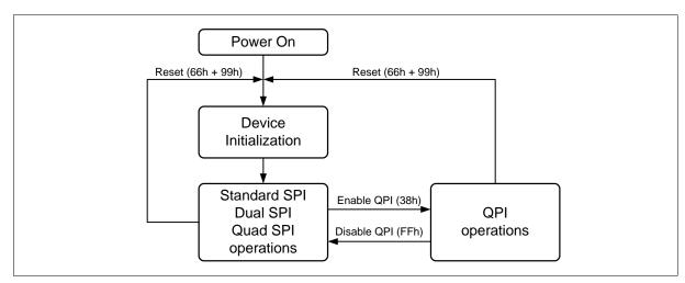
Figure 2 FM25F005A Serial Flash Memory Operation Diagram
