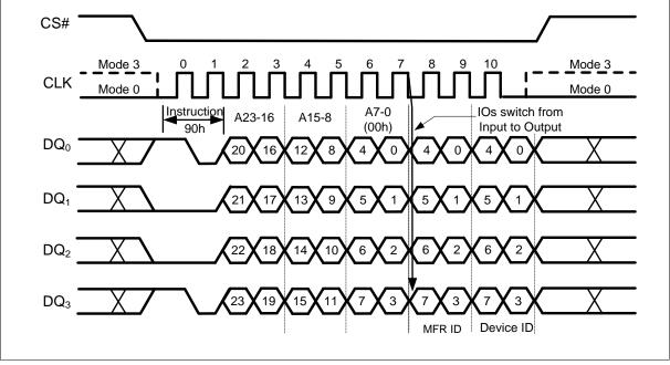
Figure 50 Read Manufacturer / Device ID Instruction (QPI Mode)
