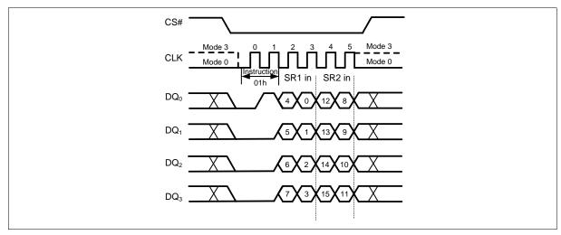
Figure 17 Write Status Register-1/2 Instruction (backward compatible, QPI Mode)
