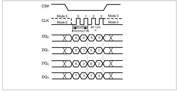
Figure 15 Write Status Register Instruction (QPI Mode)
