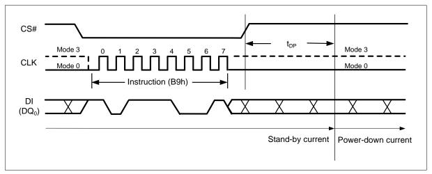
Figure 43 Deep Power-down Instruction (SPI Mode)
