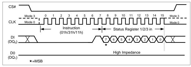
Figure 14 Write Status Register Instruction (SPI Mode)
