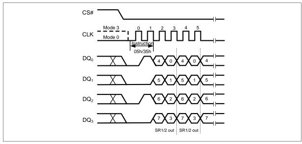
Figure 11 Read Status Register Instruction (QPI Mode)
