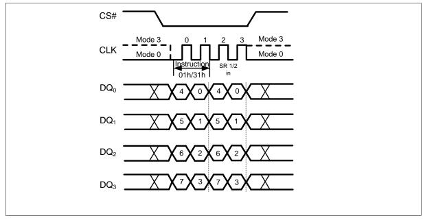
Figure 13 Write Status Register Instruction (QPI Mode)
