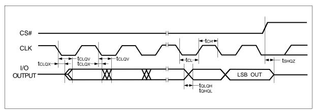
**Figure 64 Serial Output Timing**
