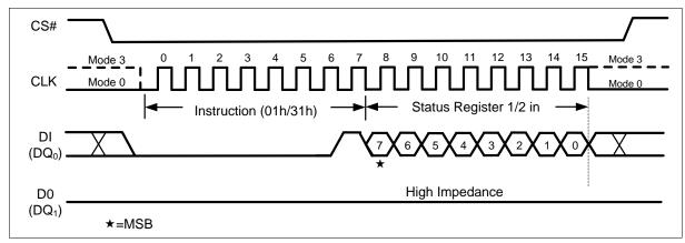
Figure 12 Write Status Register Instruction (SPI Mode)
