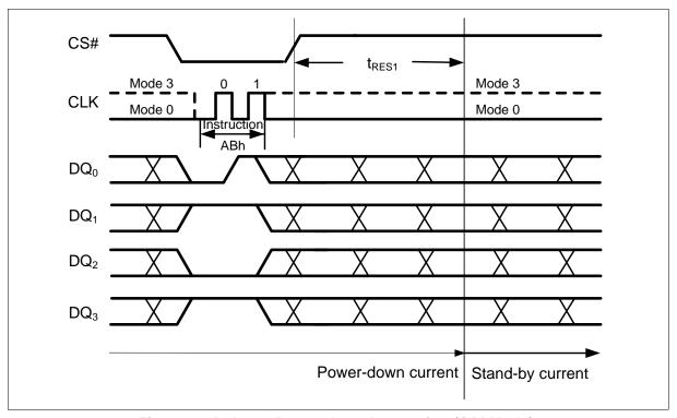
Figure 42 Release Power-down Instruction (QPI Mode)
