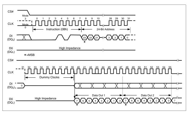
Figure 15 Fast Read Instruction (SPI Mode)
