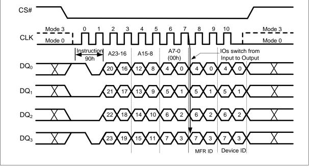
Figure 46 Read Manufacturer / Device ID Instruction (QPI Mode)
