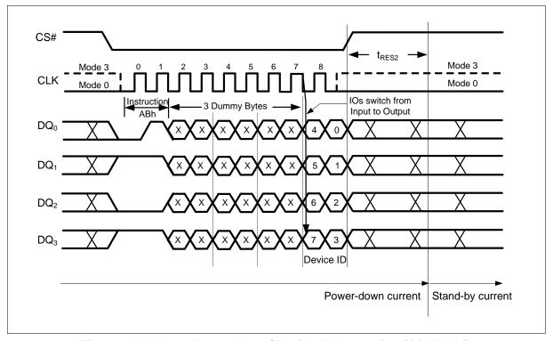
Figure 44 Release Power-down / Device ID Instruction (QPI Mode)
