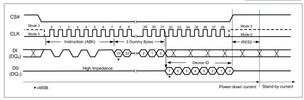
Figure 43 Release Power-down / Device ID Instruction (SPI Mode)
