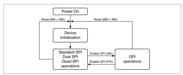
Figure 2 FM25Q04B Serial Flash Memory Operation Diagram
