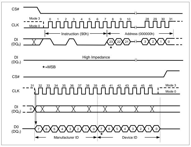
Figure 45 Read Manufacturer / Device ID Instruction (SPI Mode)
