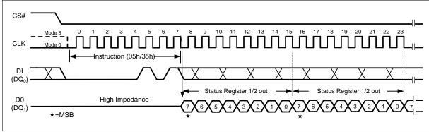
Figure 10 Read Status Register Instruction (SPI Mode)
