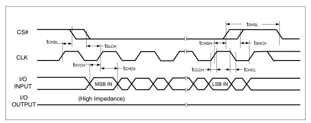
Figure 65 Serial Input Timing
