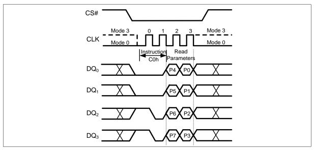
Figure 56 Set Read Parameters Instruction (QPI Mode only)
