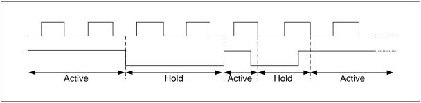
Figure 4 HoldCondition Waveform
