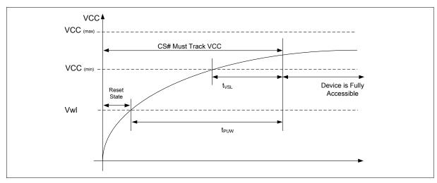
Figure 62 Power-up Timing& Power Up/Down and Voltage Drop
