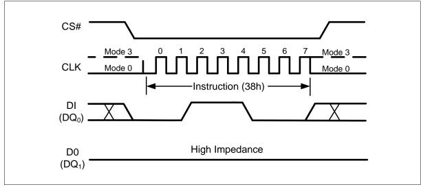
Figure 58 Enable QPI Instruction (SPI Mode only)
