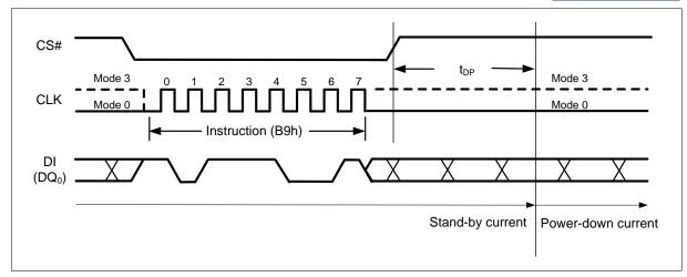
Figure 39 Deep Power-down Instruction (SPI Mode)
