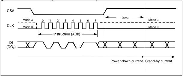
Figure 41 Release Power-down Instruction (SPI Mode)
