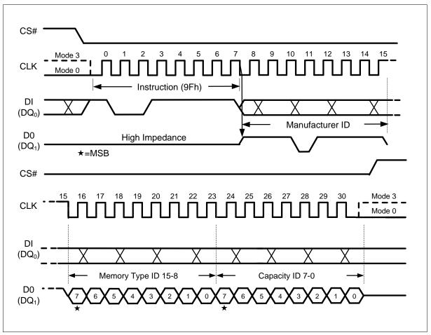
Figure 50 Read JEDEC ID Instruction (SPI Mode)
