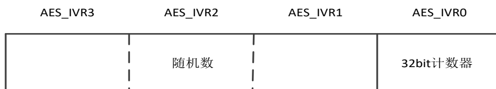
Figure 16-8 Storage Format of 32-bit Counter Value and Random Number
