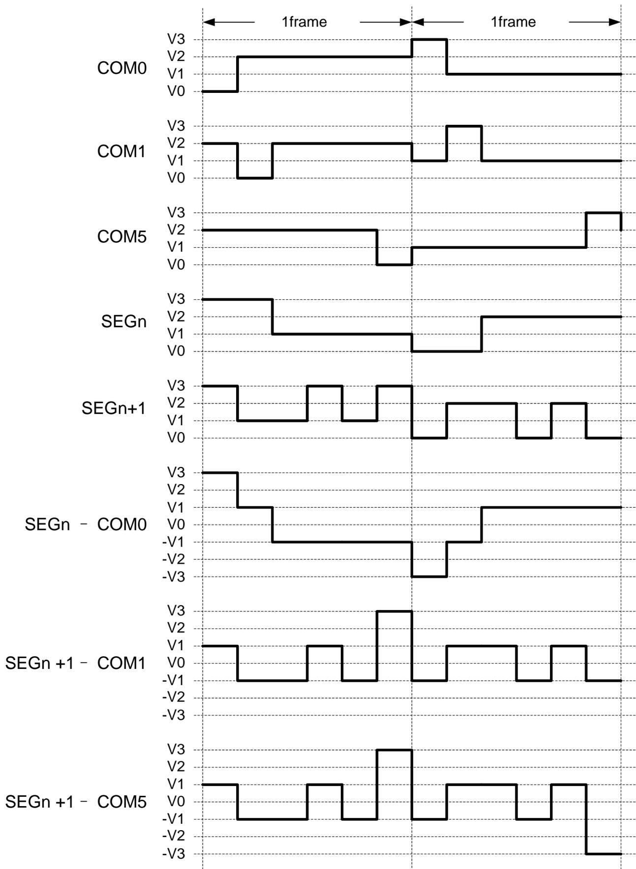
图 37-8 LCD 驱动波形(1/6 duty, 1/3 bias, type B)
