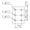
\* Dimensions of the terminals do not include thickness of pre-solder.
