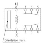
PC board mounting pad layout (TOP VIEW)
