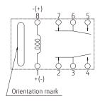
PC board mounting pad layout (TOP VIEW)
