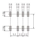
Note: Tolerance for PC board mounting hole/pad layout: +/-0.1.
