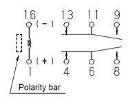
Single Coil Latching type (Top view reset position)
