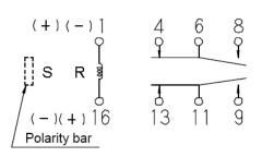
S shows the polarity of set position R shows the polarity of reset position
