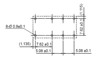
Single Coil Latching type (Bottom view reset position)
