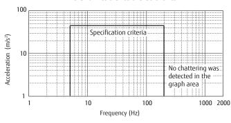
Test material: coil energized and de-energized Direction of vibration: see diagram below Detection level: chatter >1 ms
