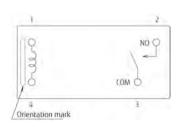
PC board mounting hole layout (BOTTOM VIEW)
