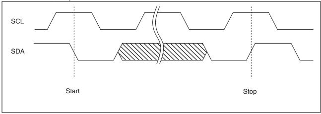
Note : The FRAM device does not need the programming wait time (twc) after issuing the Stop Condition during the write operation.
