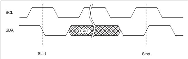
Note: At the write operation, the FRAM device does not need the programming wait time (twc) after issuing the Stop Condition.
