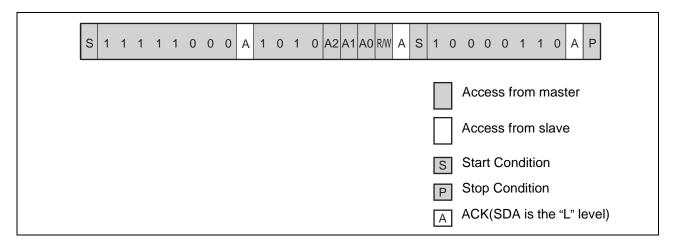
Even if the MB85RC512T stays in the Sleep mode, SDA and SCL signals are monitored. Following sequences enable the transition to Standby mode after recovery time (tree) of internal regulator circuits.
