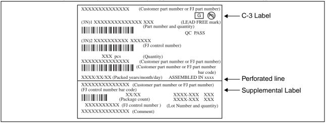
Label II: Moisture Barrier Bag (It sticks it on the Aluminum laminated bag) [MSL Label (100mm × 70mm)]
