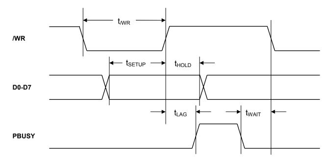
Figure 2: Parallel Interface Write Timing
