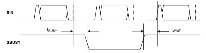
Figure 4: RS-232 Serial Interface Level Timing
