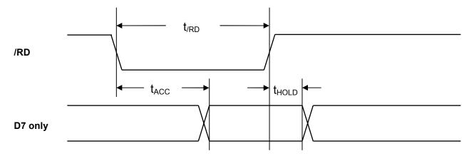
Figure 3: Parallel Interface Read Timing
