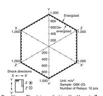
Conditions: Shock is applied in ±X, ±Y, and ±Z directions three times each with and without energizing the Relays to check the number of contact malfunctions.
