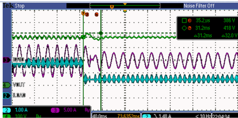
Figure 5.13. Step response 1000 -500 W at V_{Grid}=230 V: Ch.2 - i_{out} , Ch.3 - i_{Grid} , and Ch.4 - V_{out}
