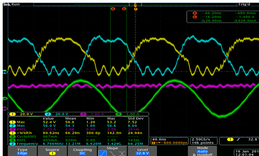
Figure 18 • Oscilloscope Plot Showing Both GS61004B Drain Node Signals
