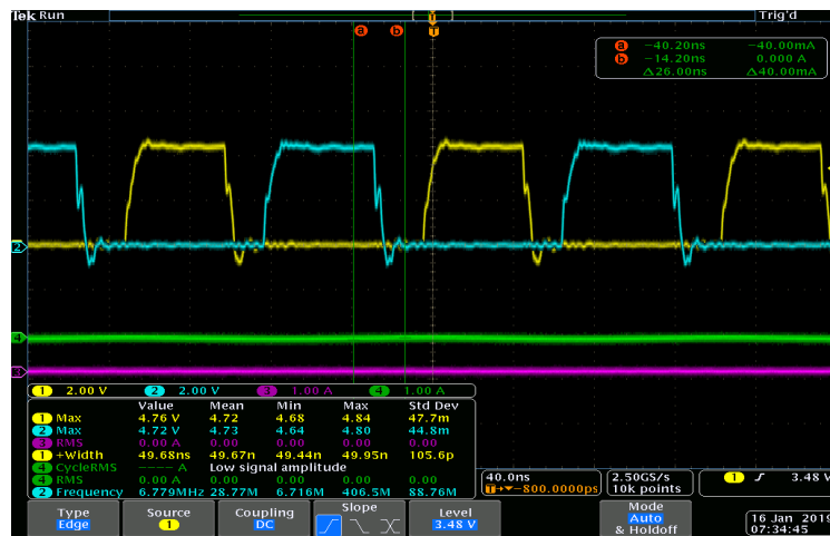
Figure 17 • Oscilloscope Plot Showing Both GS61004B Gate Node Signals at TP8, TP81
