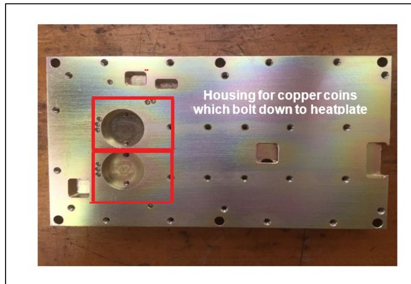
Figure 13 • Aluminum heatplate with housing for two copper coins.
