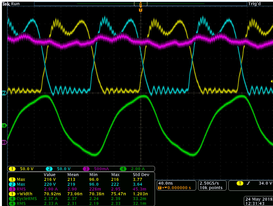
Figure 17 • Oscilloscope Plot Showing Both GS66508B Drain Node Signals, without EMI filter
