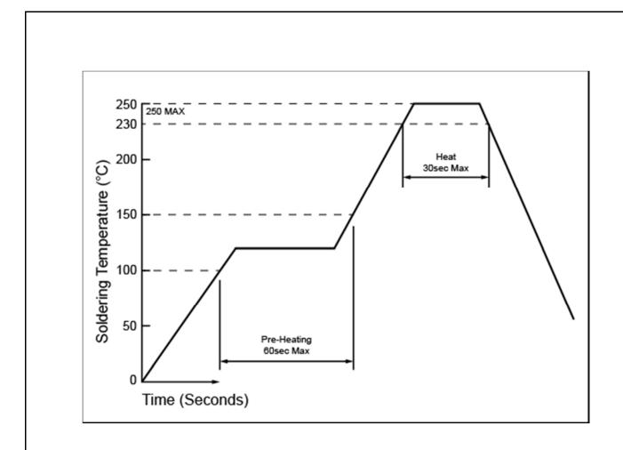
Fig. 1. Recommended Reflow Temp. Profile
