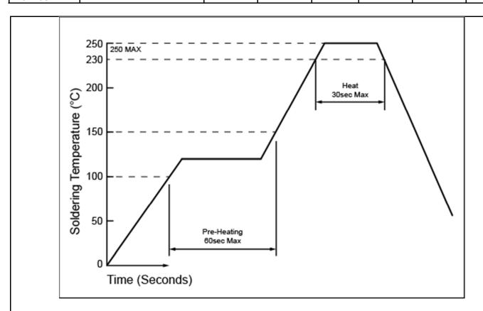
Fig. 1. Recommended Reflow Temp. Profile
