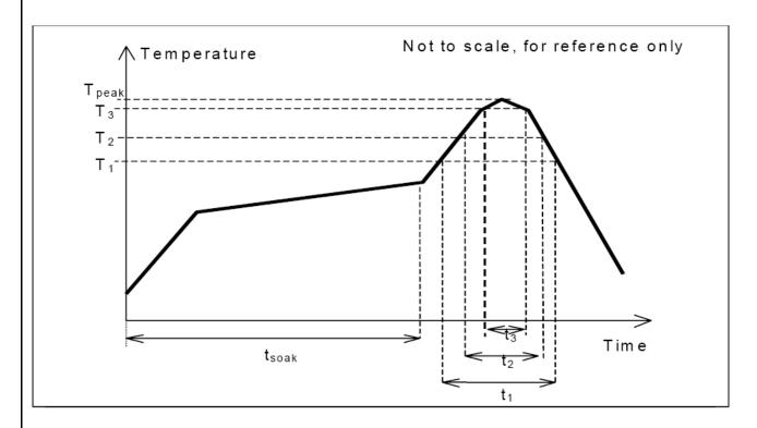
This profile is the minimum requirement for evaluating soldering heat resistance of components. Heat transfer method used for reflow soldering is hot air convection. The actual air temperatures used to achieve the specified profile is higher and largely dependent on the reflow equipment.
