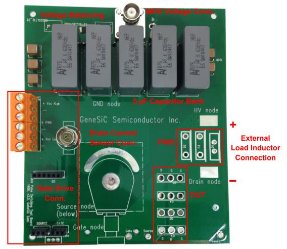
Figure 3: Switching Test Board with Labeling
