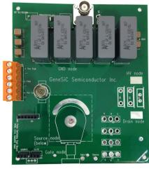
Figure 1: Double Pulse Test Board
