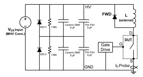
Figure 2: GeneSiC Semiconductor Switching Test Board Schematic
