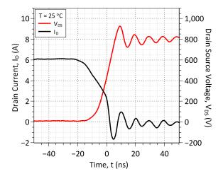
Figure 6: SJT 800V Switching Turn On Waveform
