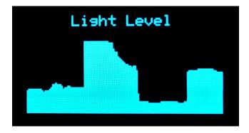
The chart is very simple. We will basically draw a vertical line that starts where the level is and ends at the very bottom of the display. The line will shift one pixel to the right in every loop.
