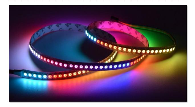
What you need to find are strips with the APA102 controller. This controller uses a SPI bus, which is available on the BrainPad. These strips are powered through different voltages. We will need 5V ones since we have access to 5V.
