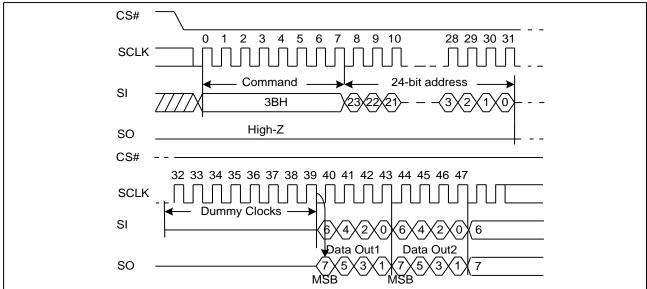
Figure10. Dual Output Fast Read Sequence Diagram
