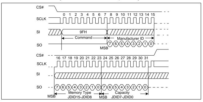
Figure28. Read Identification ID Sequence Diagram
