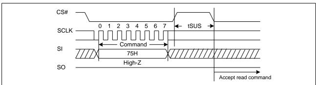
Figure29. Program/Erase Suspend Sequence Diagram
