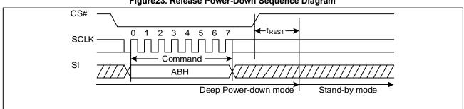
Figure23. Release Power-Down Sequence Diagram
