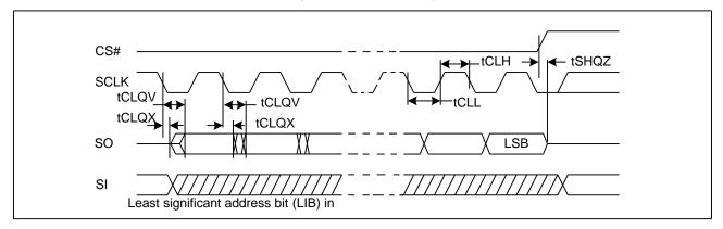
Figure42. Resume to Suspend Timing Diagram
